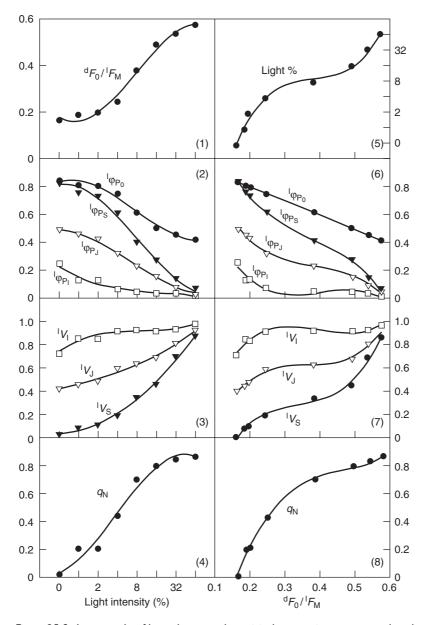
Figure 25.9 An example of how the several empirical expressions, presented vs the actinic light intensity and vs the state index  ${}^dF_0 / {}^IF_M$ , can describe the phenomenological behaviour of a sample upon light adaptation. All the curves shown here can be obtained with direct fluorescence technique (PEA, Hansatech). Usually, modulated techniques allow only measurements of curves presented with closed symbols.
