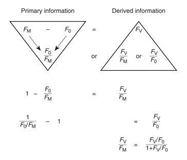
Figure 25.5 A demonstration of how the several expressions combining the extrema  $F_0$  and  $F_M$ are converted into one another.
