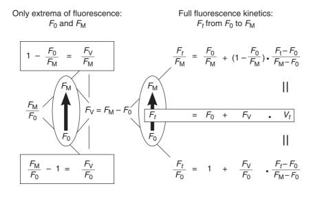
Figure 25.7 The derivation of the relative variable fluorescence  $V_t$  for an empirical quantification of the fluorescence signal. Only  $V_t$  determines the dynamic shape of any fluorescence transient.
