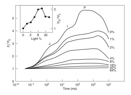
*Figure 25.3* Examples of direct fluorescence measurements with a PEA instrument. The fluorescence transients (measured with 100% light), plotted on a logarithmic time scale, were measured on pea leaves at different light adapted states (0% to 64% of 600 Wm<sup>-2</sup> for 10 sec).
