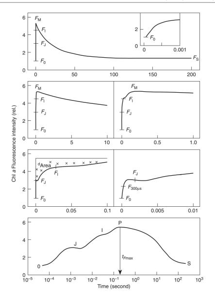
*Figure 25.1* A typical fluorescence transient exhibited upon illumination of a dark-adapted photosynthetic sample by saturating light. The transient is presented on different time scales.
