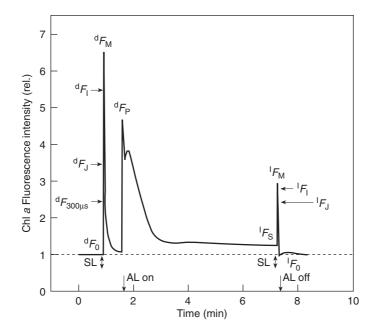
*Figure 25.2* An example of a modulated fluorescence measurement. The selected fluorescence values on the fast rise are taken from the direct fluorescence measurement of the same sample (transient of Figure 25.1). SL, saturating light; AL, actinic light.
