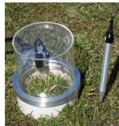
CPY-5 Canopy Assimilation Chamber
