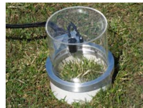
CPY-5 Canopy Assimilation Chamber
