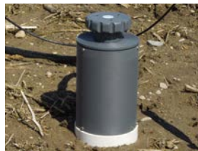
SRC-2 Soil Respiration Chamber
