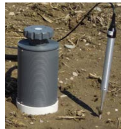
SRC-2 Soil Respiration Chamber
