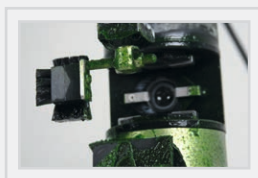
FluoroProbe III with Hydro-Wiper after weeks of operation
