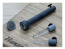
The 8 x 100mm hexagonal light guide is suited to e.g. cacti and succulents or insertion into water tanks for measurements on e.g. sea grass or coral. The light guide is protected by a sleeve and laminar samples are held in place with a magnetic puck.
