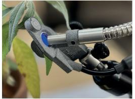
An open-faced leafclip for measurement of samples under ambient light conditions is supplied with FMS-300 as standard. The leafclip has a frontmounted PAR sensor and a leaf temperature sensor mounted within the underside of the clip. The fibre-optic is positioned at 60° to the plane of the sample and in close proximity to it. This maximises both sample illumination intensity and detection of the fluorescence signal.
