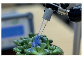
For measuring smaller samples such as Arabidopsis, needles and lichens, two tapered light guides are available. The tapered form of these light guides focuses the light from FMS-300 and increases the maximum saturating pulse intensities. The two light guides have dimensions at the sample end of 4 x 4 mm and 2.5 x 2.5 mm providing up to 60,000 and 90,000  $\mu$ mol m<sup>-2</sup> s<sup>-1</sup> respectively.
