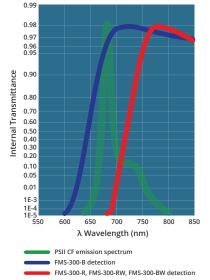
Figure 2: Detector characteristics of FMS-300 variants relative to the chlorophyll a emission spectrum.
