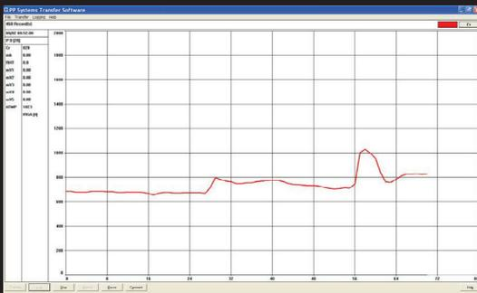
The WMA-4 is supplied with a Windows® based software program for transferring and logging sensor data. The sensor data may be recorded manually or automatically depending on user specified settings. Stored records (ASCII) can be later imported into your favorite spreadsheet program for further analysis.
