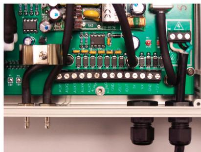
*System power, analog and digital outputs and sensor inputs are connected through the terminal blocks located inside the WMA-4 enclosure.*
