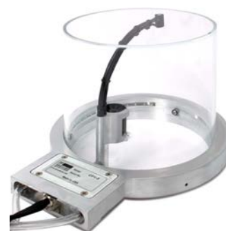
CPY-5 Canopy Assimilation Chamber Includes sensors for measurement of air temperature and PAR
