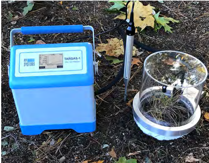
TARGAS-1 Portable Photosynthesis System shown with STP-2 Temperature Probe & CPY-5 Canopy Assimilation Chamber
