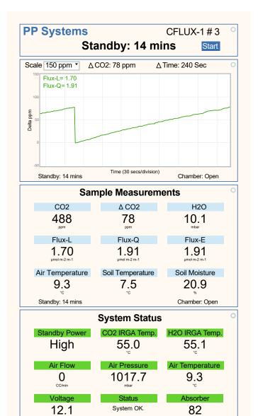
Sensor data and information is easily viewed via computer or mobile device. Flux rates based on linear and quadratic fit are continuously calculated and displayed.
