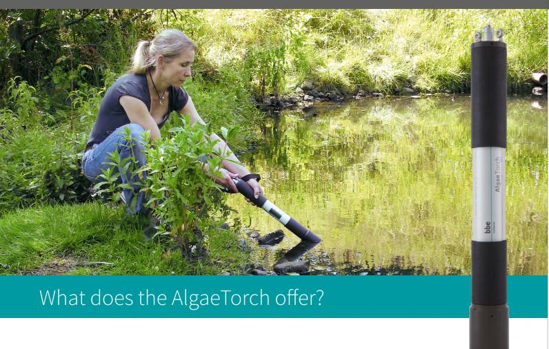
The AlgaeTorch is a handheld instrument for the rapid measurement of chlorophyll-a without sample preparation.
