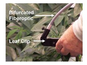
For most customers interested in typical leaf reflectance measurements, we recommend the following system configuration (including optional external battery pack for extended use in the field:
