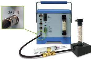
**NOTE:** The column must remain vertically oriented throughout the process.
