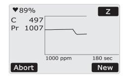
The IRGA pressure (**Pr**) is displayed to help identify when gas is pushed into the EGM-5 too quickly causing overpressure and unstable readings. Use a slow and steady stroke to keep the pressure near ambient.
