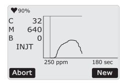
Typically during an injection, the first value will rise quickly and drop back to zero; correspondingly, the value of M will increase quickly as the value of C, then plateau at a constant value. Once C has dropped to 0 ppm (or a very low background value), wait 3-5 seconds to make sure M has stabilized and take note of the value. NOTE: If using a USB memory stick, the value will automatically be recorded.
