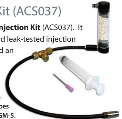
The injection port includes a 9 mm low-bleed septum that can withstand up to 50 injections (per the manufacturer's specification) and a guide hole that will accommodate up to a 22-gauge syringe.
