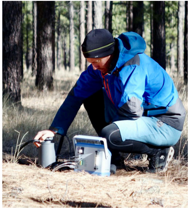
Figure 3: Andrew Abraham and Chris Doughty take measurements of soil respiration using a PP Systems EGM-5 Portable CO 2 Gas Analyzer in one of their 0.25 ha plots near Flagstaff, Arizona.
