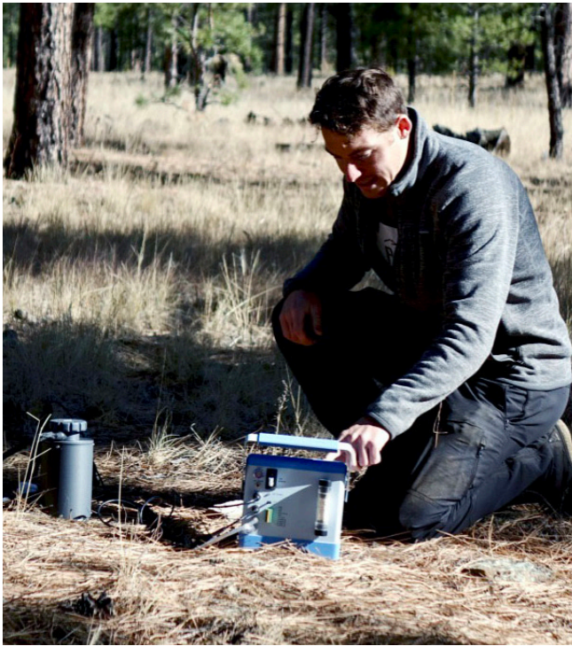
Figure 3: Andrew Abraham and Chris Doughty take measurements of soil respiration using a PP Systems EGM-5 Portable CO 2 Gas Analyzer in one of their 0.25 ha plots near Flagstaff, Arizona.
