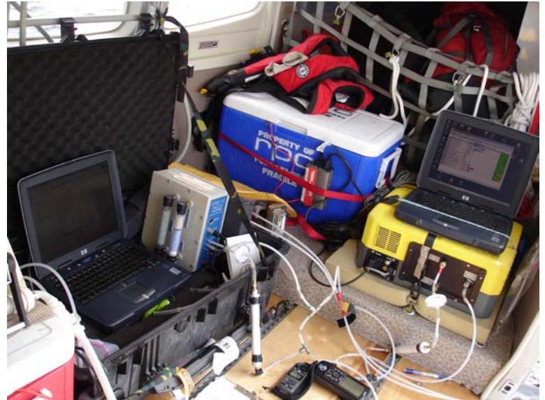
Figure 3. Suite of research instrumentation including the CIRAS-SC used to determine near-surface GHG fluxes in combination with the floating chamber.
