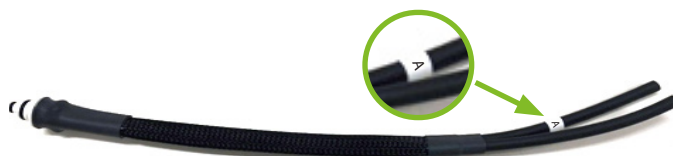
Leaf Cuvette Simulator with "Y" piece and single gas line removed.
