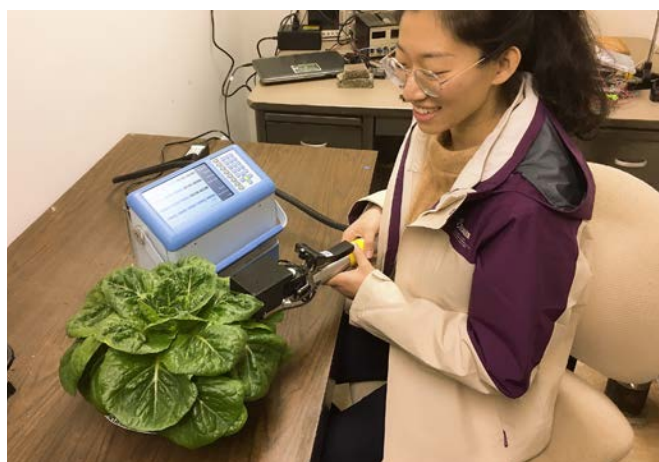
Jun Liu, Ph.D. student under Dr. Marc van Iersel, taking photosynthetic measurement with the CIRAS-3 Portable Photosynthesis System.
