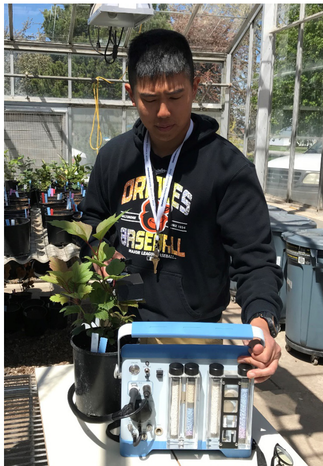
Fig. 1. Ji-Jhong Chen, master student under Dr. Youping Sun, recorded the gas exchange data of viburnums using the CIRAS-3 Portable Photosynthesis System.
