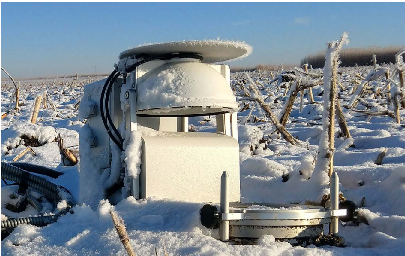
A CFLUX-1 Automated Soil CO 2 Flux System shown in early December 2018 after snowfall.
