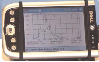
PP Systems has developed new software that will allow you to operate your UniSpec from a PDA. The software has been developed and thorougly tested on a Dell Axim PDA that features Microsoft Windows Mobile OS v5 and a virtual VGA (640 x 480) resolution screen.
