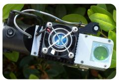
Close-up of PLC4 (B) leaf cuvette head
