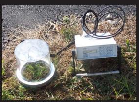
The CPY-4 shown above with the EGM-4 Environmental Gas Monitor for CO<sub>2</sub>
