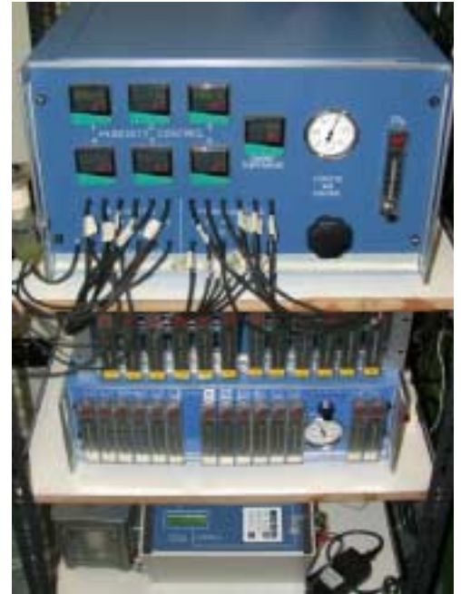
Close-up view of CIRAS-1 gas analyzer, gas switching unit and environmental control system.
